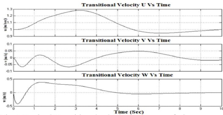
Fig 6: Desired Transitional velocity responses of tri-copter.
