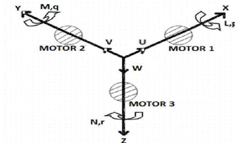
Fig 1: 120-degree Phase Typical Diagram of Tri-Rotor Vehicle.
