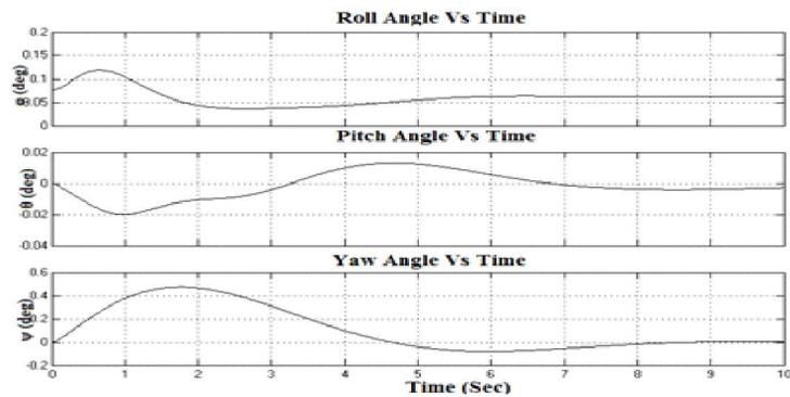
Fig 5: Desired Euler angle responses of tri-copter.
