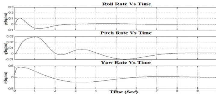
Fig 4: Desired Angular Rate responses of tri-copter.
