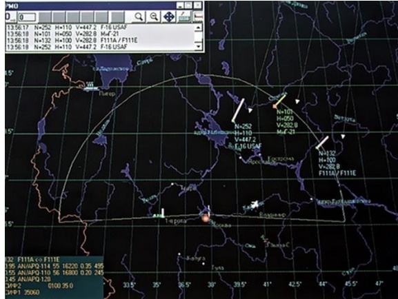
Fig. 5. Mapping display of lantan/almaz-antey valeria elint and emitter Locating System
