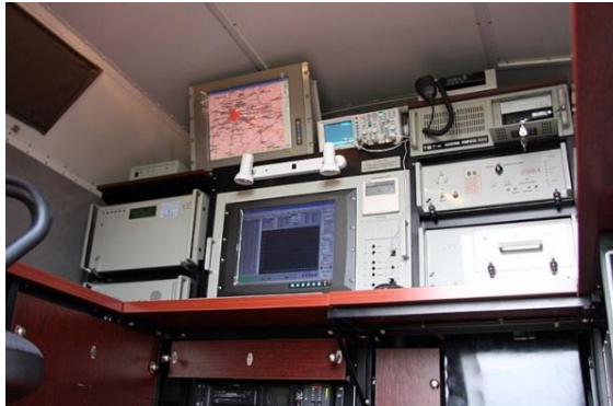
Fig. 6. Topaz Kolchuga direction estimation system consoles
